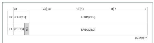
Fig 137. Extended message ID filter element
