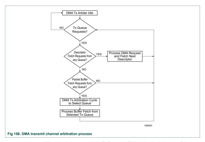
When there is any request in the Tx Queue, the DMA arbiter checks the type of the request: packet buffer fetch or descriptor fetch request. The descriptor fetch requests have higher priority than the buffer requests. Therefore, when there is a descriptor fetch request, the DMA arbiter acknowledges the DMA channel that is requesting for a descriptor fetch. If there is no descriptor fetch request, the arbiter looks for packet buffer fetch requests.
