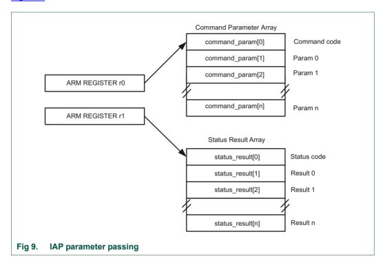
The number of parameters and results vary according to the IAP command. The maximum number of parameters is 5, passed to the "Copy RAM to flash" command. The maximum number of results is 5, returned by the "ReadUID" command. The command handler sends the status code INVALID\_COMMAND when an undefined command is received. The IAP routine resides at location 0x0300 0204 and is in ARM Thumb code, therefore called as 0x0300 0205 by the Cortex-M4 to insure Thumb operation.
