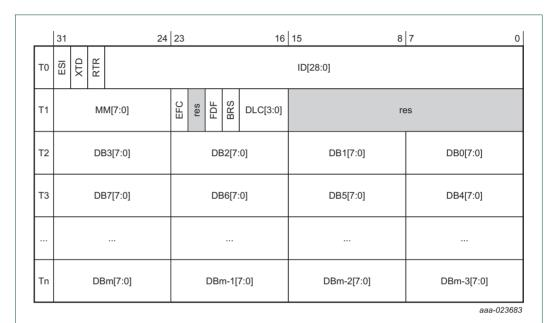
Fig 134. Tx buffer element
