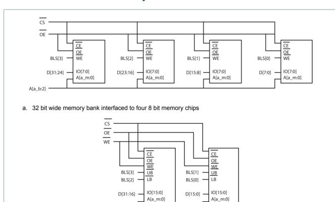
b. 32 bit wide memory bank interfaced to two 16 bit memory chips
