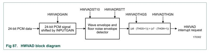
Because of the non-uniqueness of the input signal, which includes normally noise and voice with various frequency components and different volume, there is no one-and-only operation mode for the HWVAD. The few parameters as well as the chronology can play an important role for a good performance.
