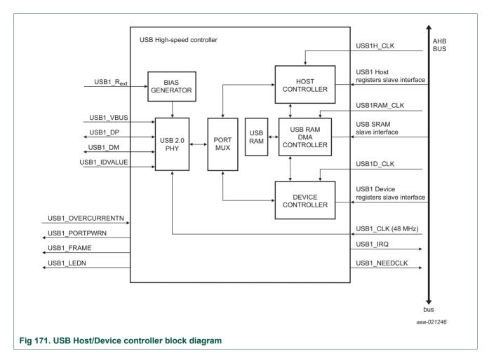
The USB device controller has a built-in analog transceiver (PHY). The USB PHY sends/receives the bi-directional USB1 DP and USB1 DM signals of the USB1 bus.
