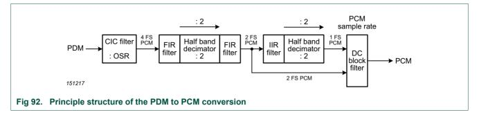
To achieve lower power consumption, the DC filter can be supplied with the 2FS instead of the 1FS signal, bypassing the second half band decimator filter. This reduces the required DMIC base clock by a factor of 2. This is done by setting the USE2FS bit in the USE2FS register.
