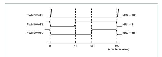
Fig 46. Sample PWM waveforms with a PWM cycle length of 100 (selected by MR3) and MAT3:0 enabled as PWM outputs by the PWCON register.
