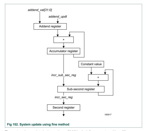
The system time update logic requires a 50 MHz clock frequency to achieve 20 ns accuracy. The frequency division is the ratio of the reference clock frequency to the required clock frequency. Hence, if the reference clock is, for example, 66 MHz, this ratio is calculated as 66 MHz / 50 MHz = 1.32. Hence, the default addend value to be set in the register is  $2^{32}$  / 1.32, 0xC1F07C1F.
