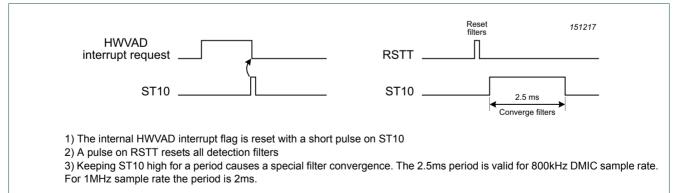
Fig 88. Use of ST10 and RSTT controls (in the HWVADST10 and HWVADRSTT registers)
