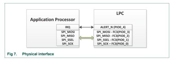
A typical transaction starts with the host writing a command packet and the LPC546xx device processing the command packet. It asserts the ALERT\_N line LOW when processing is complete and then the host system can read the response packet. The device will dessert ALERT\_N pin whenever the host starts a new transaction, that is, as soon as SPI\_SSEL goes active. See <a href="Figure 8">Figure 8</a>.
