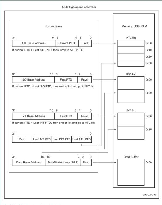
Fig 177. USB host software interface
