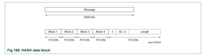
The ARM processor uses little-endian and therefore, the Hash block reverses the bytes in the words written to the data register to big-endian format. This is because a Hash is on bytes, so a string such as "abcd", when read as a word by the processor (or DMA) is reversed into "dcba". When the input data is provided in little-endian format, the Hash block swaps them to process correctly.
