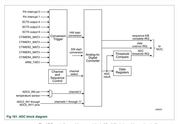
The ADC controller provides a great deal of flexibility in launching and controlling sequences of ADC conversions using the associated 12-bit, successive approximation ADC converter. ADC conversion sequences can be initiated under software control or in response to a selected hardware trigger.
