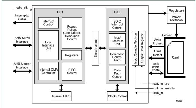
Note: The Card Detect and Write Protect signals are from the SD/MMC card socket, not the SD/MMC card itself.
