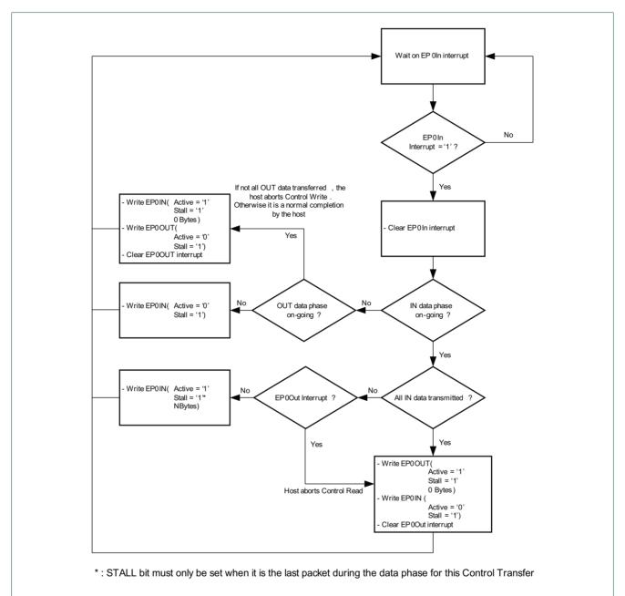
Fig 169. Flowchart of control endpoint 0 - IN direction
