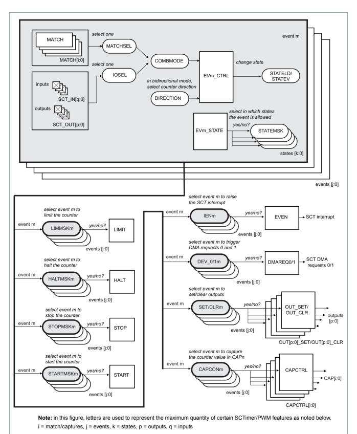
Fig 36. SCTimer/PWM event configuration and selection registers
