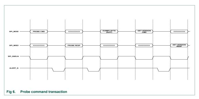
In  $I^2C$ , when this dummy byte is sent from the host via an  $I^2C$  write operation, do not send a  $I^2C$  read operation to check for any response. After the dummy byte write operation, the host system can follow the  $I^2C$  ISP mode transaction protocol as discussed in following sections.
