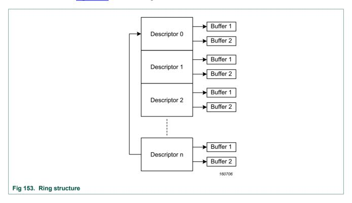
The transmit and receive engines enter the running state and attempt to acquire descriptors from the respective descriptor lists. The receive and transmit engines then begin processing receive and transmit operations. The transmit and receive processes are independent of each other and can be started or stopped separately.
