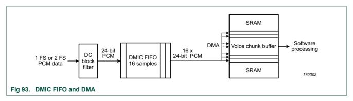
The 24-bit wide FIFO of the DMIC interface consists of 16 entries for each of the two channels. The trigger level for the FIFO can be set in register FIFOCTRL[0:1] individually for each channel.
