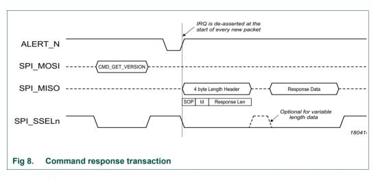
Although SPI is bidirectional, the command and response packet phases only sends data one way for each phase. During the command packet phase, the host system should ignore the read data (sent from the LPC546xx device).
