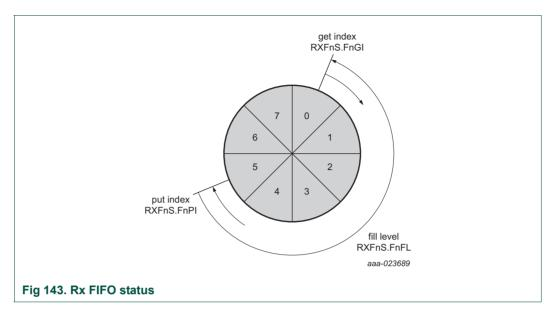
When reading from an Rx FIFO, the Rx FIFO get index bit field in the Rx FIFO status register \* FIFO element size has to be added to the corresponding Rx FIFO start address in the Rx FIFO configuration register.
