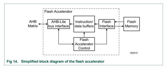
In the following descriptions, the term "fetch" applies to an explicit flash read request from the CPU. "Prefetch" is used to denote a flash read of instructions beyond the current processor fetch address.
