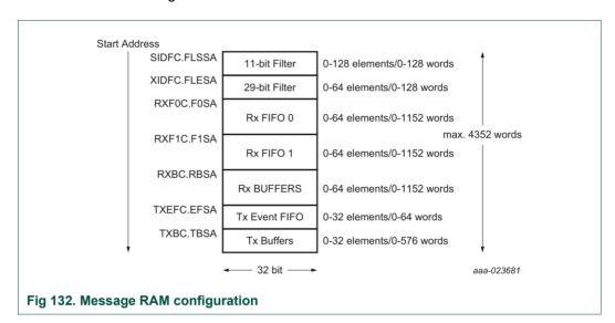
When the MCAN module addresses the message RAM, it addresses 32-bit words, not single bytes. The configurable start addresses are 32-bit word addresses, that is, bits 15 to 2 are evaluated, the two least significant bits are ignored.
